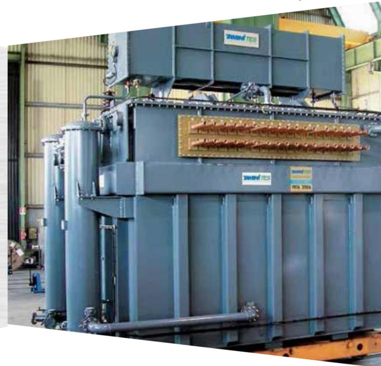
steel melting process. Continuous stresses and vibrations might make the windings loose if they are not properly treated and robustly clamped. In order to avoid any inconvenience due to such heavy and frequent stresses, Tamini has adopted improved procedures for windings pressing and thermal treatment operation.
