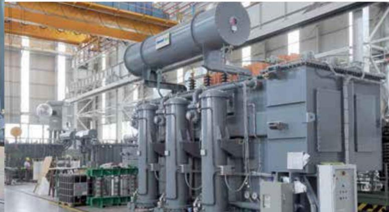
The coolers can be equipped with many accessories line: water and oil flow indicators with alarm contact, water and oil thermometers, water and oil drain taps or other special ones, on request. When water is not available, the cooling is generally OFAF.
